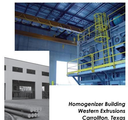
Three buildings were designed by RWA at the complex, the first of which was the Homogenizer Building, where 14"-diameter "logs" of aluminum are heated to increase their suitability for extrusion. The open-air structure houses the homogenizer which rolls over the stack of logs, heats the material, and then rolls away to heat a second stack, while the first cools. The other buildings we designed on the site are a warehouse and a two-story tilt-wall shipping office.
